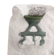
Oxide colour after divesting with traditional NiCr alloy
