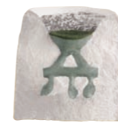
Oxide colour after divesting with Wiron® light
