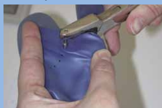
Punching of holes at the marked positions
