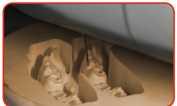
Milling a saw-cut model with the 3D model-disc 100
