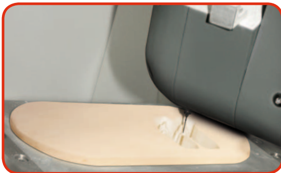
Swivel unit with mounted circular blank holder for 3D model-disc XL
