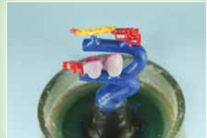
Invest OT UNILATERAL and Uni-Box in one step into casting ring. For best results, use an alloy with 240 Vickers.
