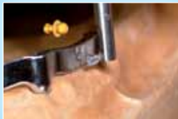
Apply a two part composite to the shank of the sphere. Using the tool, insert the sphere into the hole. Wait for the composite to cure.
