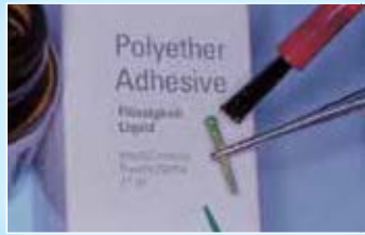
Apply adhesive to the post.
